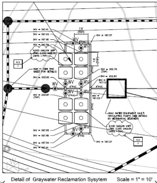
At the Roger L. Putnam Regional High School, stormwater runoff from a section of rooftop will be captured in a series of cisterns for use in flushing all toilets and urinals. Roof drainage will be collected in four 4,000 gallon underground tanks that direct flow to the school's gray water plumbing system. The project also includes a raingarden, grass swale, and a series of infiltrators. These facilities are capturing stormwater from the parking area.
